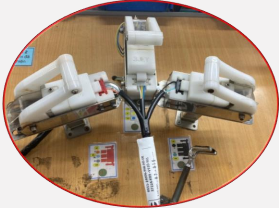
Fitting of Terminal and Connector Jig Check
